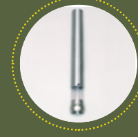
Metal soil sampling cylinder (50-100 mm length, 1.6 mm gauge wall, and 75-100 mm in diameter with both ends open)
