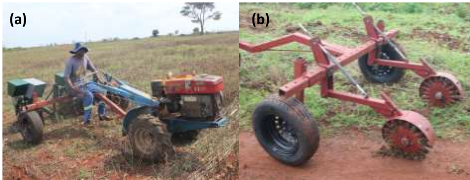
Figure 1 – (a) wheeled toolbar on which two planting units (manufactured by Grownet) are attached; and (b) two starwheels attached to a toolbar.
