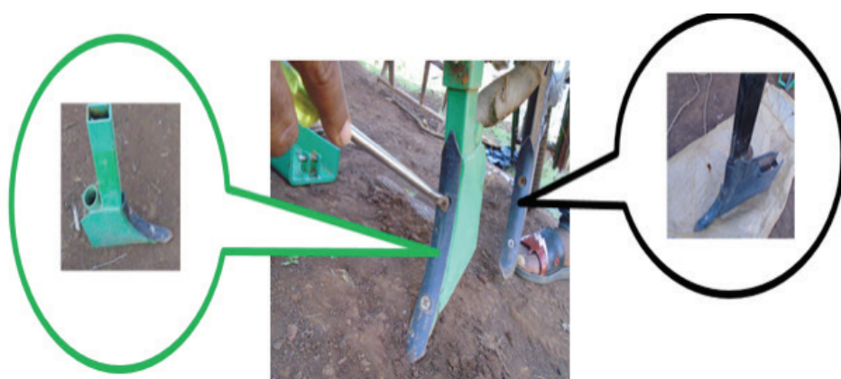
Fig 61. Furrow opener, the green one is furrow opener for fertilizer while the black one is for seed.
