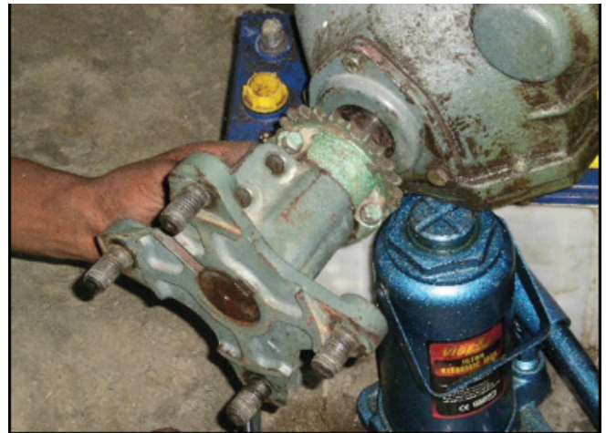
Fig 49. Removing the flange of the axle and inserting the drive sprocket to the drive axle.
