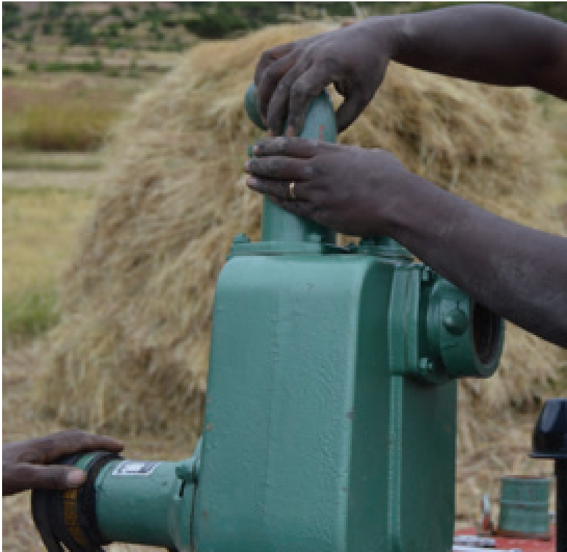
Fig 89 & 90. Inserting the elbow in the discharge side (top of the pump).
