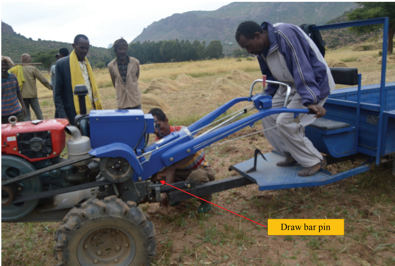
Fig 72. Separating the trailer from the 2WT.
