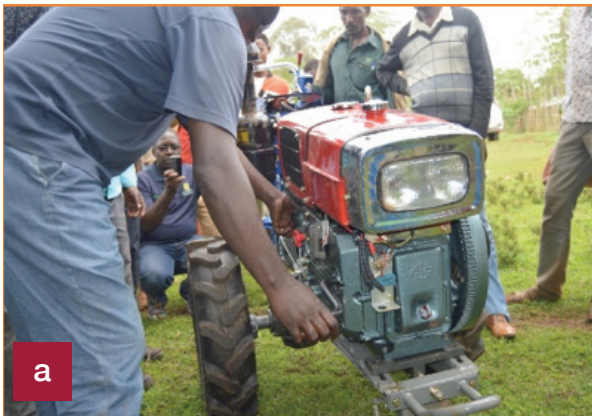
Fig 14. 2WT manual starting (a) and electrical starting (b).
