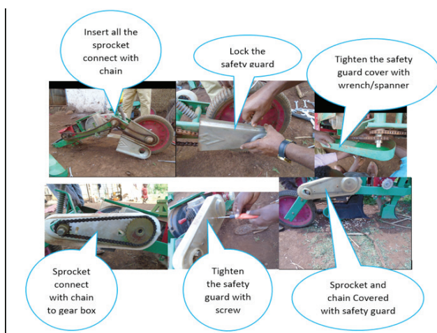
Fig 67. Assembling of metering unit.
