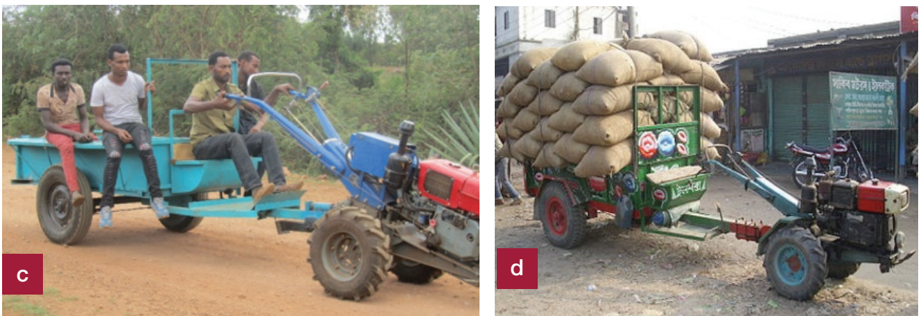
Fig 9. 2WT application for transportation(c) 1ton trailer at Gudeya Bila, Oromia Region, Ethiopia (d) 5 t trailer in Bangladesh.
