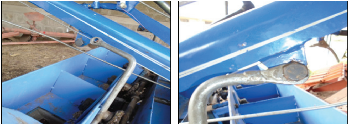
Fig 47. Mounting levers to attach the VMP to the 2WT steering column.
