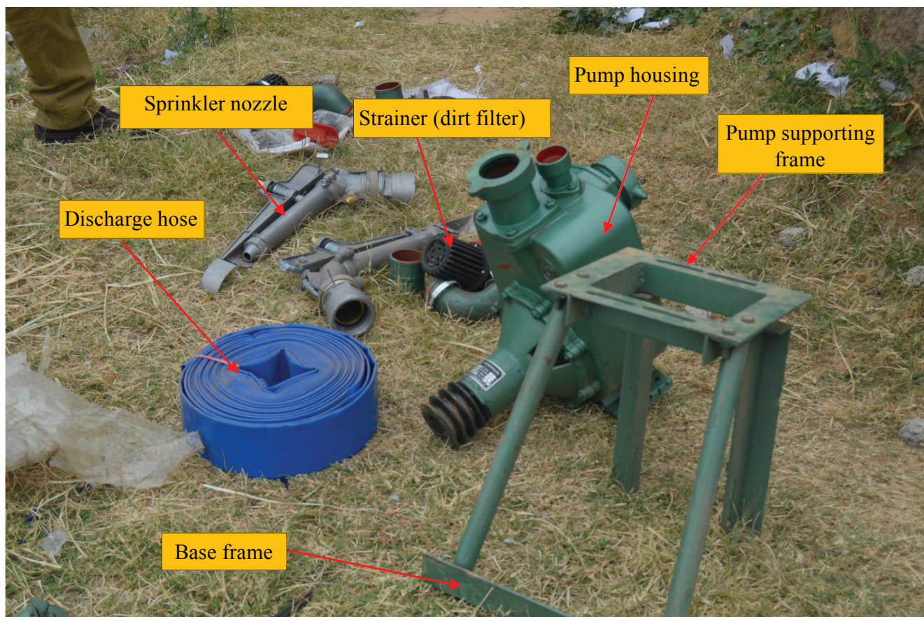
Fig 75. Complete set of 2WT attached water pump.
