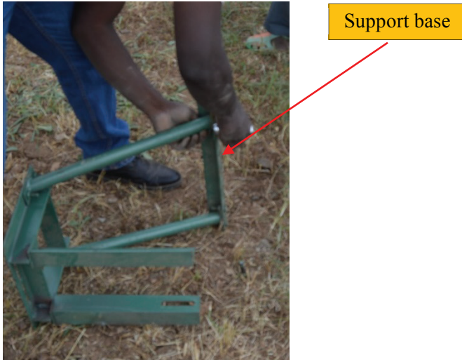
Fig 76. Removal of the securing bolts.
