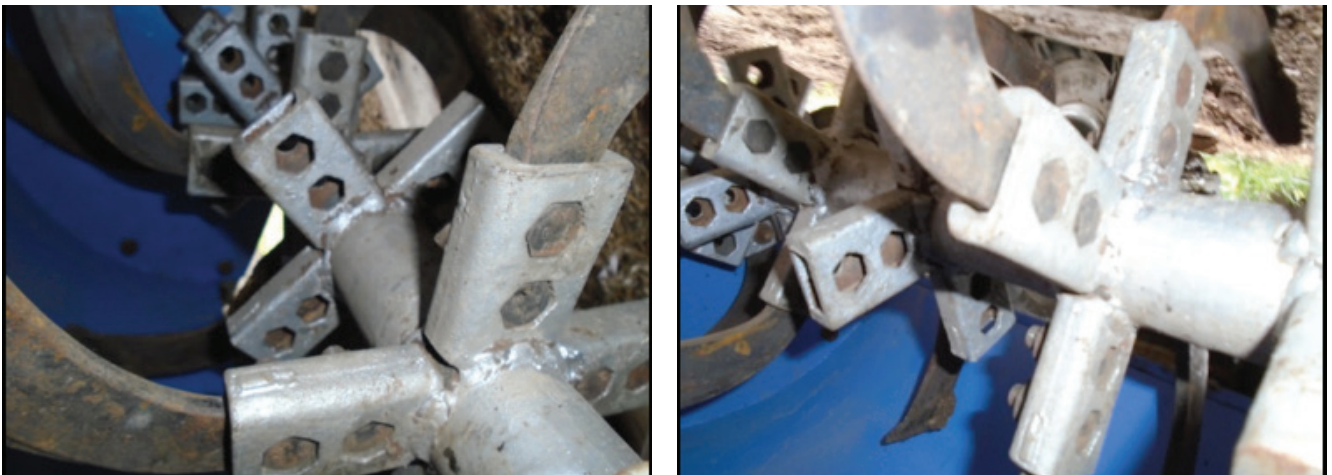
Fig 43. Ripping blades on the rotavator shaft.
