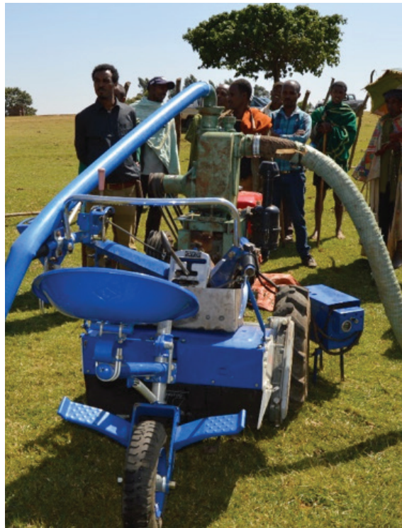
Fig 6. 2WT application for water pumping for irrigation (a) Machakel District, Amhara Region and (b) Adwa district, Tigray Region, Ethiopia.
