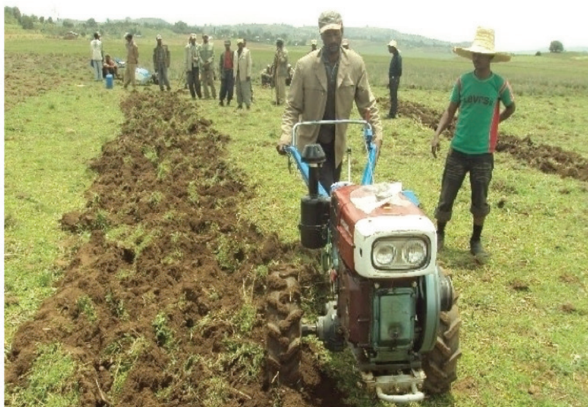
Fig 3. 2WT application for ploughing (at Wolmera District, Oromia Region, Ethiopia) In planting/seeding different crops.
