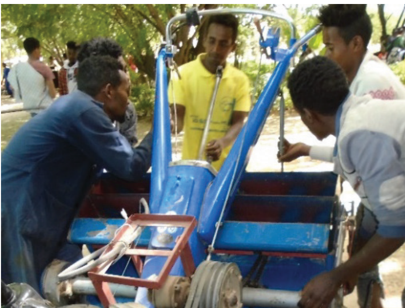
Fig 26. Mounting levers to attach the VMP to the 2WT steering column.
