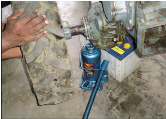
Fig 48. Lifting the wheel with a hydraulic jack
