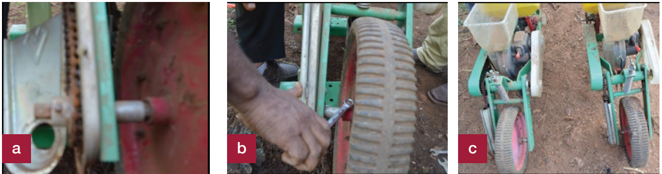
Fig 68. Drive wheel assembly a): Inserting drive wheel, b): Tightening the securing bolt and c): Assembled drive wheel.
