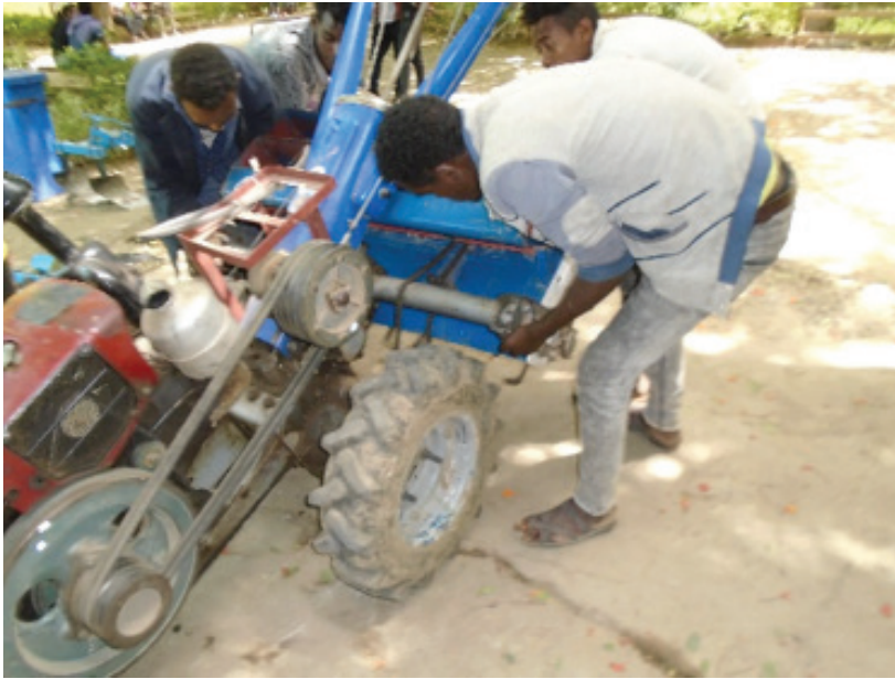
Fig 25. Mounting the 2BFG-100 to the drawbar pull/gearbox of the 2WT.
