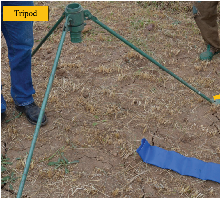
Fig 91. Fix the tripod on the ground using the black pins using your foot or any other hammering tool.
