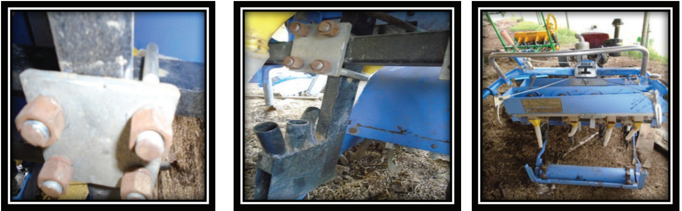
Fig 42. Furrow opener and assembling hinge with u-bolts.
