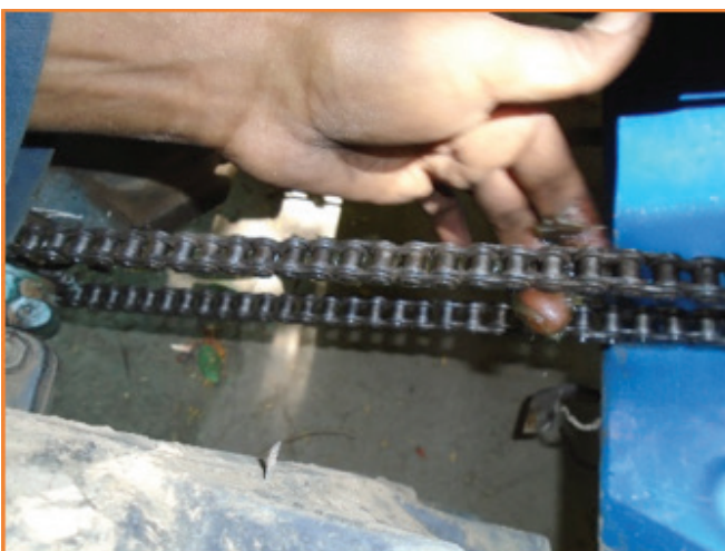
Fig 29. Lubricating the chain and sprocket.
