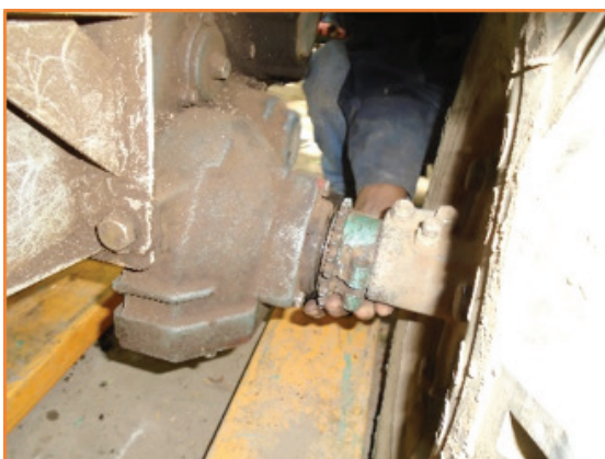
Fig 20. Inserting the drive sprocket to the drive axle.
