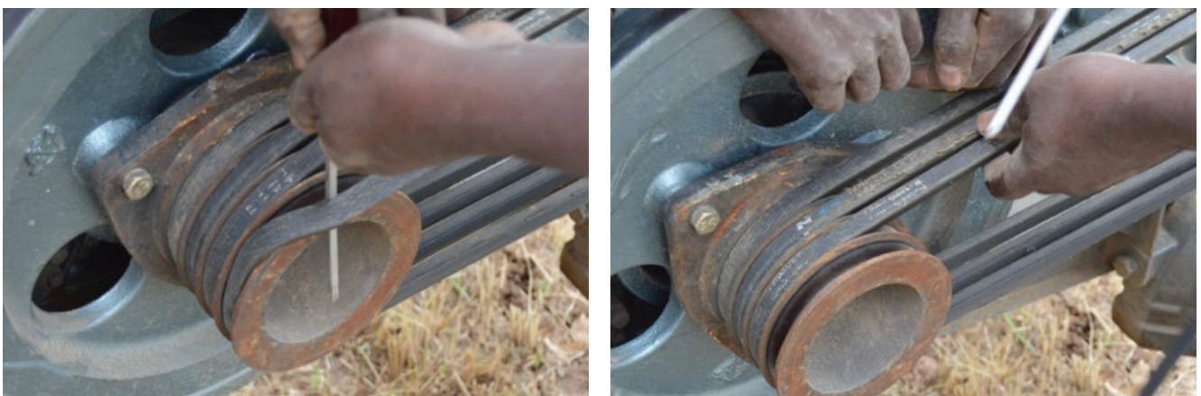
Fig 81 & 82. Removing the v-belts from the engine crankshaft pulley.
