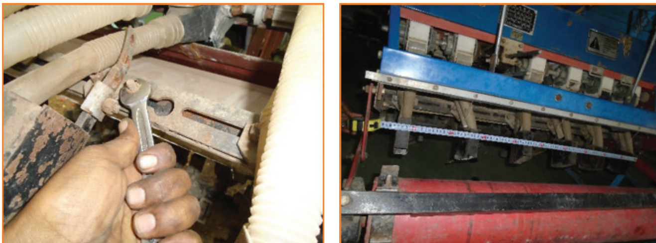
Fig 21. Assembling of furrow openers.
