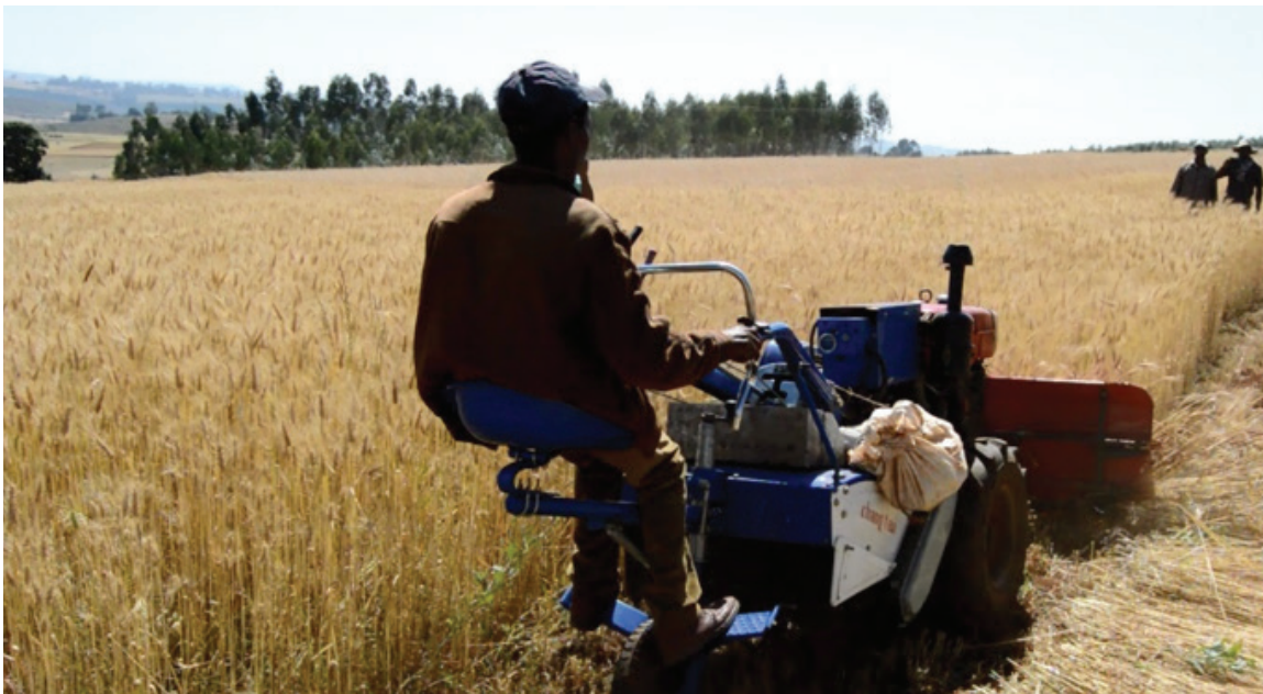
Fig 7. 2WT application for harvesting (Wheat harvesting in Machakel district, Amhara Region, Ethiopia).
