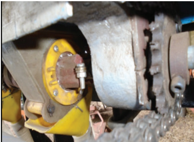
Fig 50. Assembled sprocket and chain drive.
