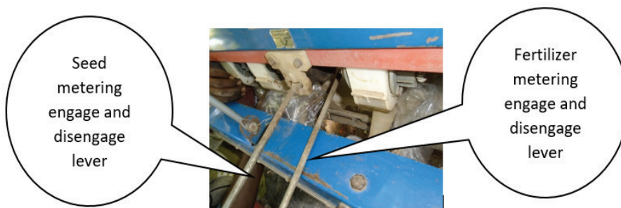
Fig 32. Seed and fertilizer metering engage and disengage lever.
