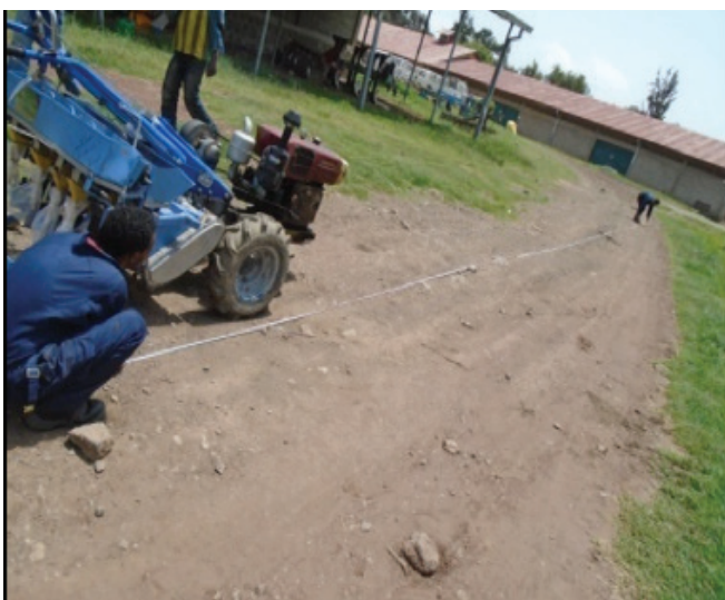
Fig 52. Measuring 30 meters for calibration.
