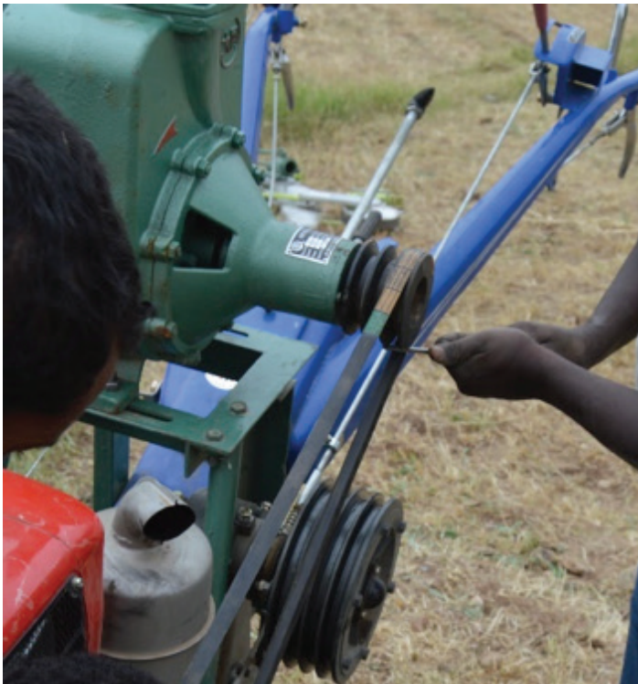
Fig 83. Inserting a v-belt from the engine pulley side and then from the clutch pulley.
