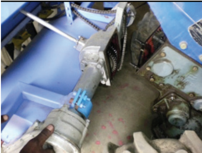
Fig 46. Mounting the VMP to the drawbar pull of the 2WT.
