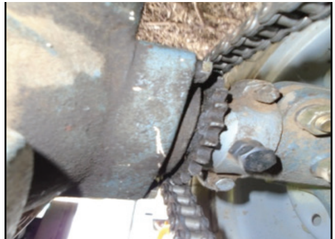
Fig 49. Removing the flange of the axle and inserting the drive sprocket to the drive axle.
