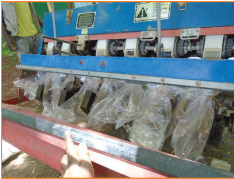
Fig 34. Attaching transparent polythene bags to each of the six seed delivery tubes.
