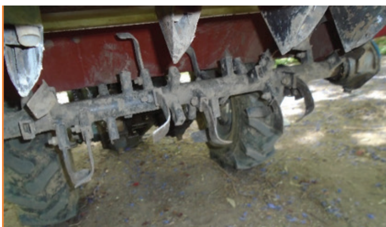
Fig 22. Installed blades on the rotavator shaft.
