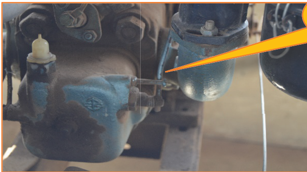
Fig 16. 2WT decompression knob.
