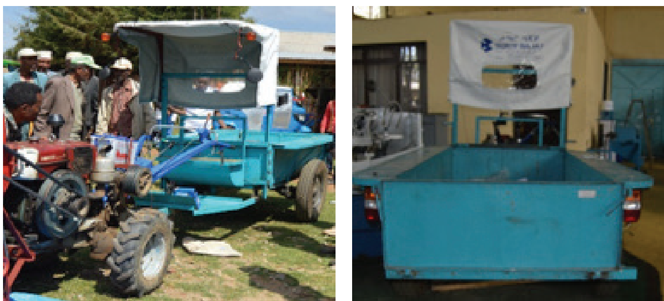
Fig 104. Modified 1000 kg capacity trailer to be use on roads made by EIAR through FACASI phase-II project (demonstrated during field day at Tiyo District, Oromia region, Ethiopia).
