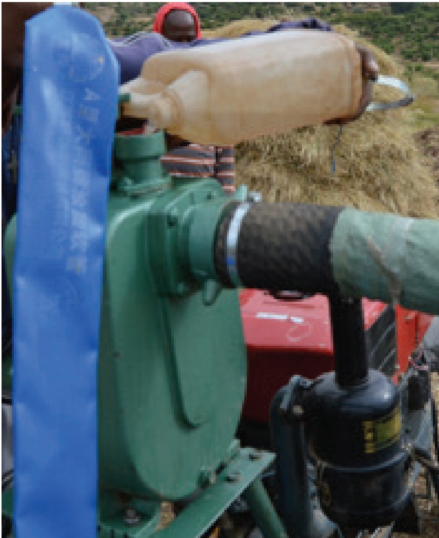
Fig 97. Fill water at the right top of the pump until it is full (priming).
