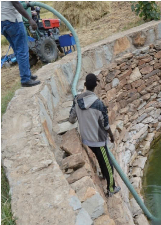
Fig 6. 2WT application for water pumping for irrigation (a) Machakel District, Amhara Region and (b) Adwa district, Tigray Region, Ethiopia.
